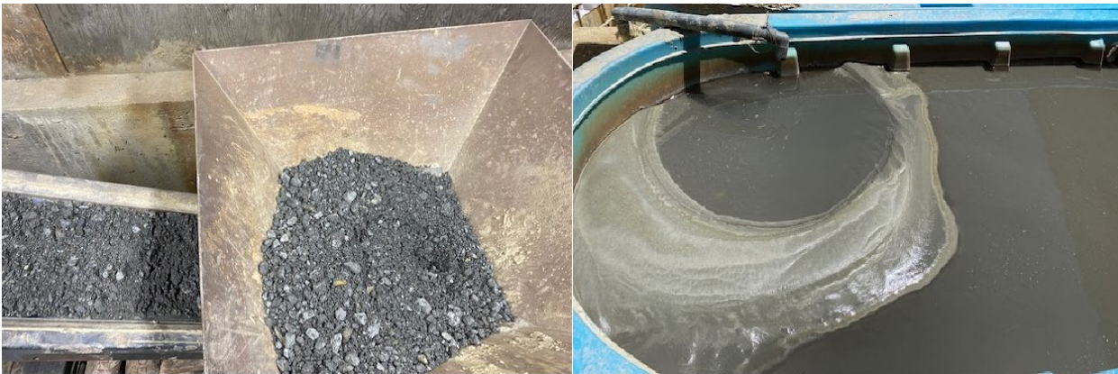
Figure 1: Crushed Ore in Hopper and Conveyer (ball mill feed)
